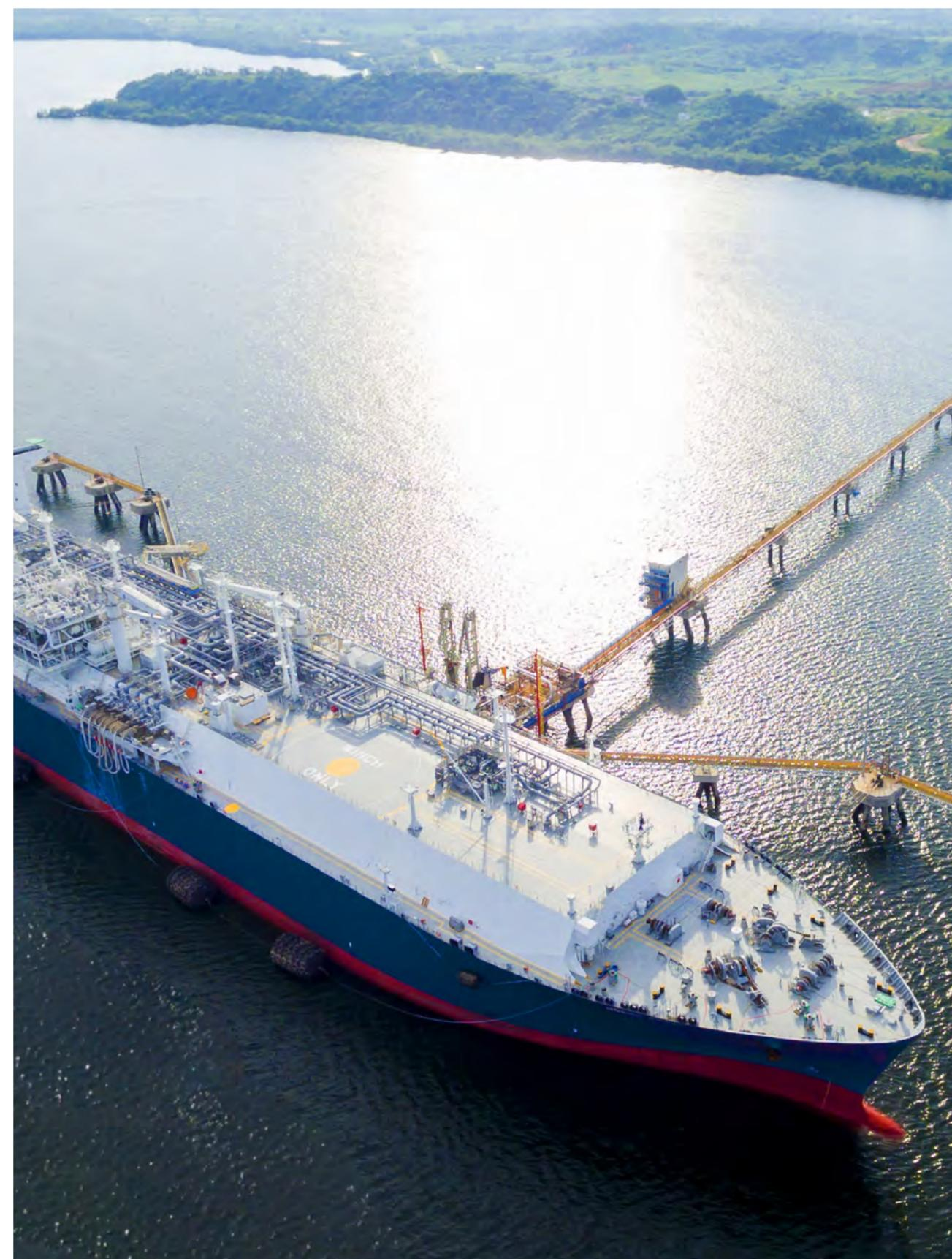
FSRU Based - LNG Terminal - Courtesy of SPEC LNG
