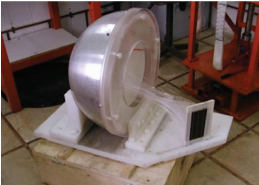
**Figure 8.** Model of an experimental system in the Nuclear Archive representing what appears to be a shock wave generator and high explosive, with a diagnostic system using fiber optic cables, to measure time of arrival of a detonation front in the main charge.
