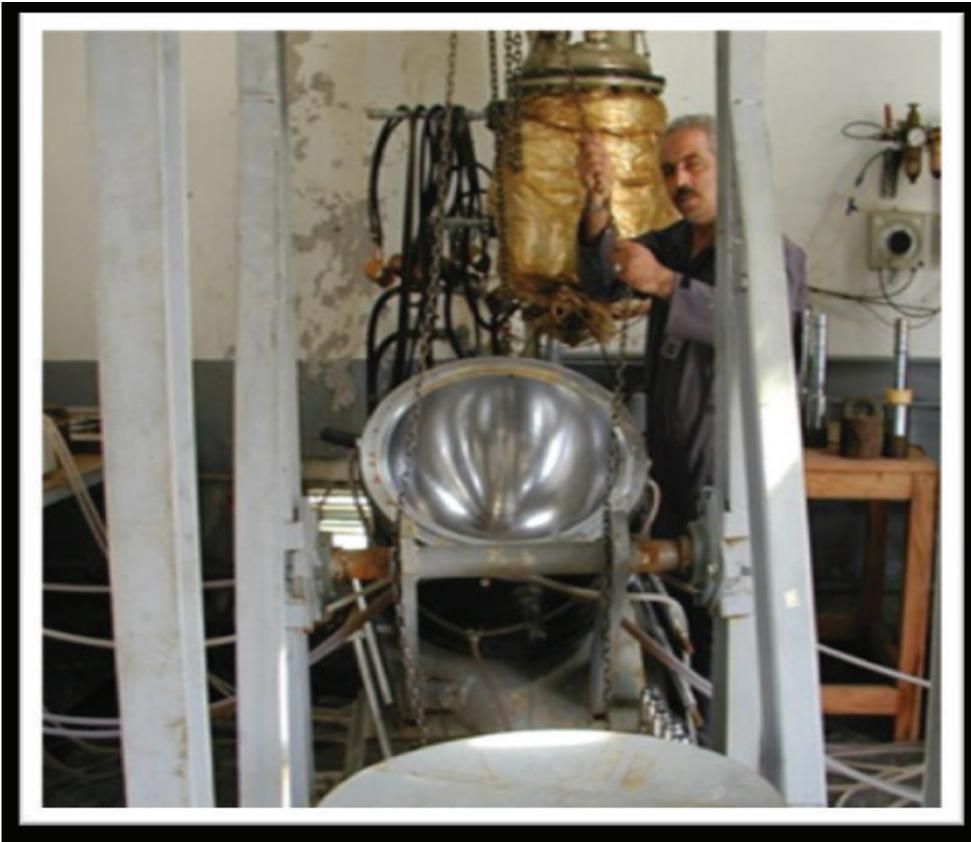
**Figure 3.** Image from the Nuclear Archive that shows a high high-explosive casting mold at an unidentified location in Iran. The equipment in the background could not be identified.
